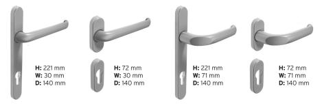
A handle with a long cover plate or a short cover with cylinder cover and a long grip. Ideal for roll down shutters. A handle with a long or short cover plate and a long grip. A cylinder cover is also available.
